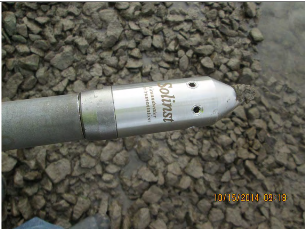
Photo 7: Solinst® Drive Point Profiler – pore water sampling device
