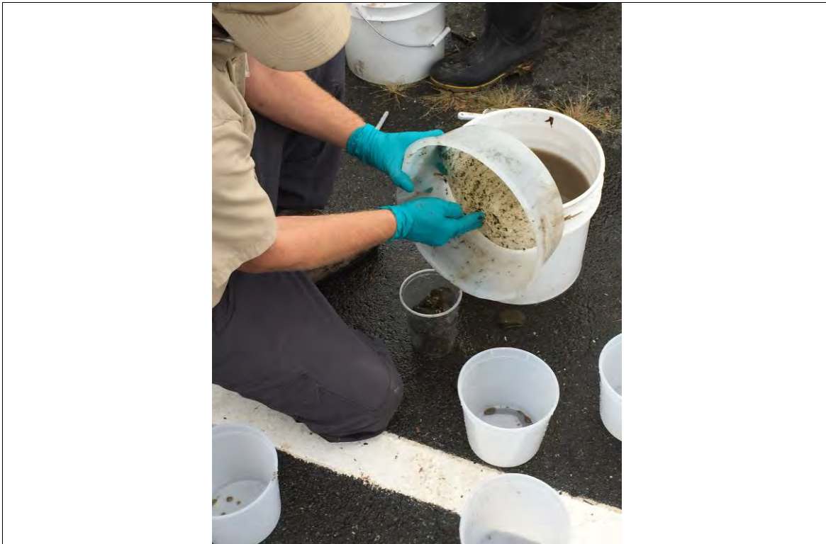
Photo 10: 500-micron sieve used for biological sample collection
