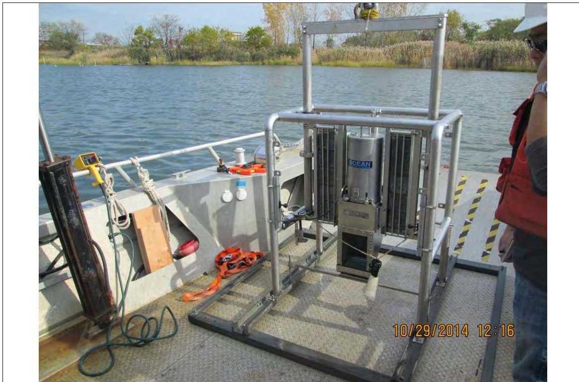
Photo 13: SPI Camera staged on deck of vessel
