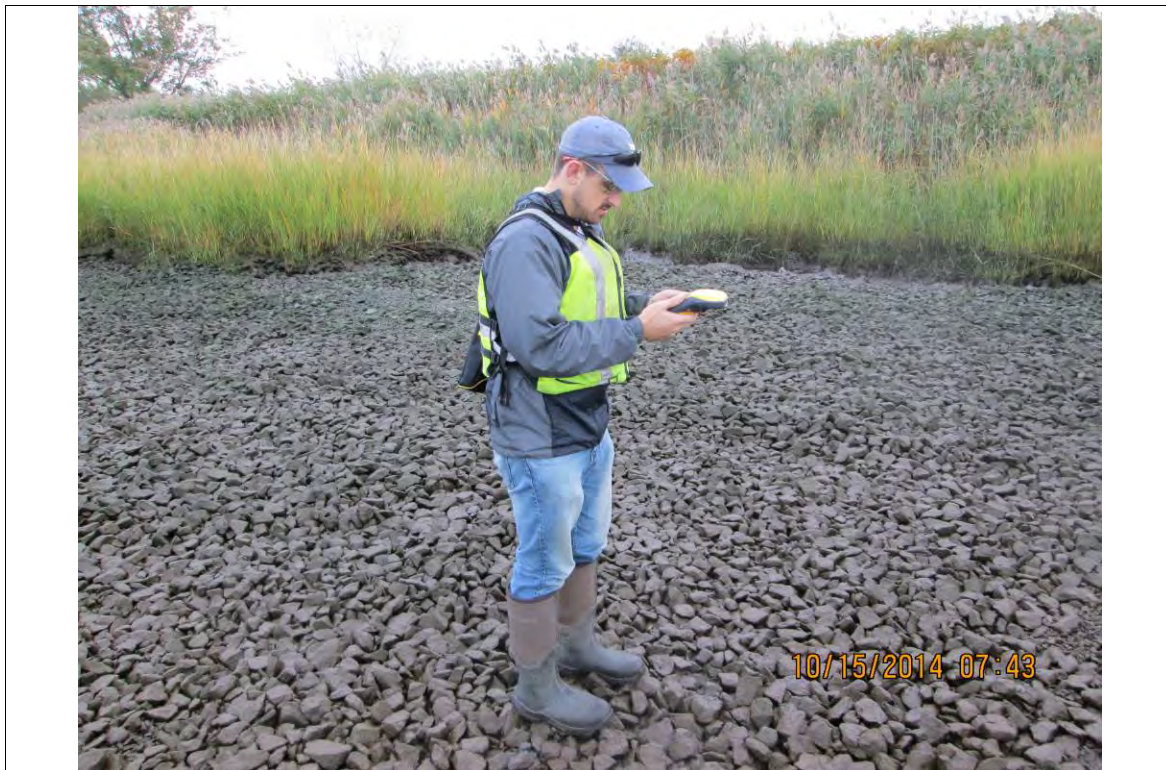
Photo 2: Navigation to intertidal long-term monitoring plate location using Trimble SPS855 GPS unit
