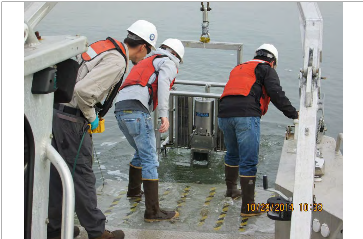
Photo 14: Deploying the SPI Camera in subtidal MNR area
